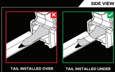
D. When hooking a new Tape Blade on, make sure to have the Power Spring Tail attach from underneath the new Tape Blade, and ensuring that both sides of the Power Spring Tail are wrapped around the top of the Tape Blade.
