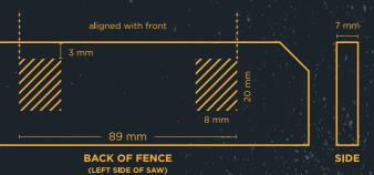
Ribs may be thicker as M1 clamp can extend to clear these ribs while moving device to suitable clamping position
