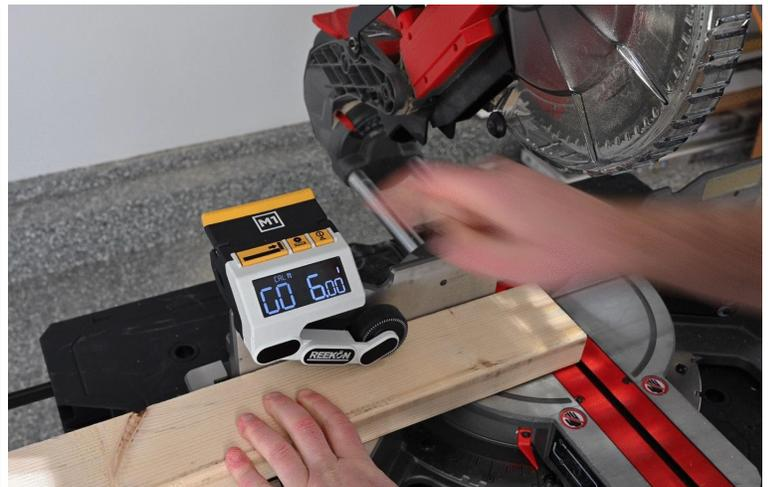
4. Move material slightly to the right and ensure the material is stable on saw setup and select units (ft or m)
